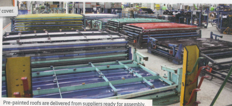
Pre-painted roofs are delivered from suppliers ready for assembly.
