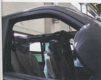
The roof has already been cut out during the build on the main factory assembly line.
