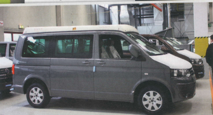
Vehicles come from the Hannover factory fitted with a temporary rigid plastic roof cover.
